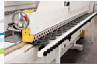
Disc roller side support Special for narrow work piece.
