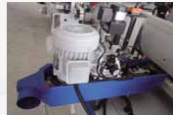
PS7: Belt sanding unit Sanding Motor: 2HP Sanding belt size: 4"x 60" Vibration power: 25w x 1/36
