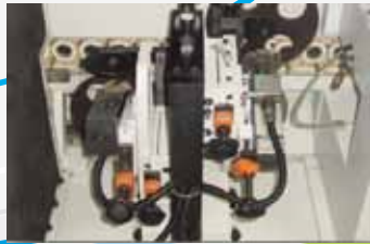
ET2 : Tilting edge trimming unit Apply for fine trimming of top and bottom edge as "chamfering". Spindle tiltable : 0 ~ 35° Cutters : 80 x 20 MM / 100 x 20 MM Speed : 12000(50HZ) / 14400 (60HZ) R.P.M. Motors : 0.5 HP x 2 / 1.8 HP x 2 / 2.5 HP x 2 Space required : 645 MM
