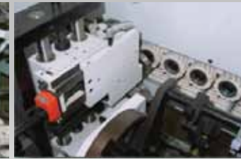
LS1 : Longitudinal cutting shear Apply for longitudinal cutting shear of top and bottom of soft forming edges. (for SD-700A)
