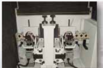
PM1 : Profile moulding unit PM(left hand) / PM2(right hand) Apply moulding on panel edge or lipping. Standard with H.F. motors. Spindle tiltable : 0 ~ 180° Cutter : 80 x 20 MM / 120 x 30MM Speed : 12000(50HZ) / 14400(60HZ) R.P.M Motor : 2.5 HP / 5 HP Space required : 570 MM
