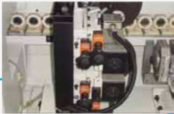
ET1 : Edge trimming unit Apply for rough trimming of top and bottom edges. Cutters : 80 x 20 MM Speed : 12000(50HZ) / 14400 (60HZ) R.P.M Motors : 0.5 HP x 2/1.8 HP x 2/2.5 HP x 2 Space required : 455 MM
