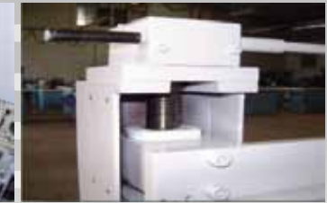
The top pressure beam equipped with ball screw transmission
