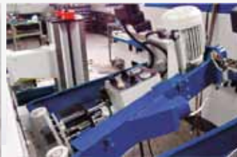
PS5 : Profile sanding unit PS5(left hand) / PS6 (right hand) Apply sanding on profile edge. Spindle tiltable : -15 ~ + 105° Belt size : 4" x 78" / 98" Belt speed : 630 MM Motors : 2 HP Space required : 750 MM
