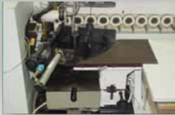
EGL3 : Double gluing unit Apply glue on panel and/or edge "Soft forming" also applicable. Glue pot : 7KG Power : 4 KW Space required : 580 MM
